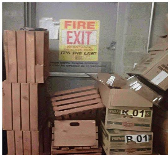
Picture 2 shows a poorly stored materials and supplies room. It is hard to move around, it is unclear if there are any fire extinguishers. The whole situation poses a serious fire risk
